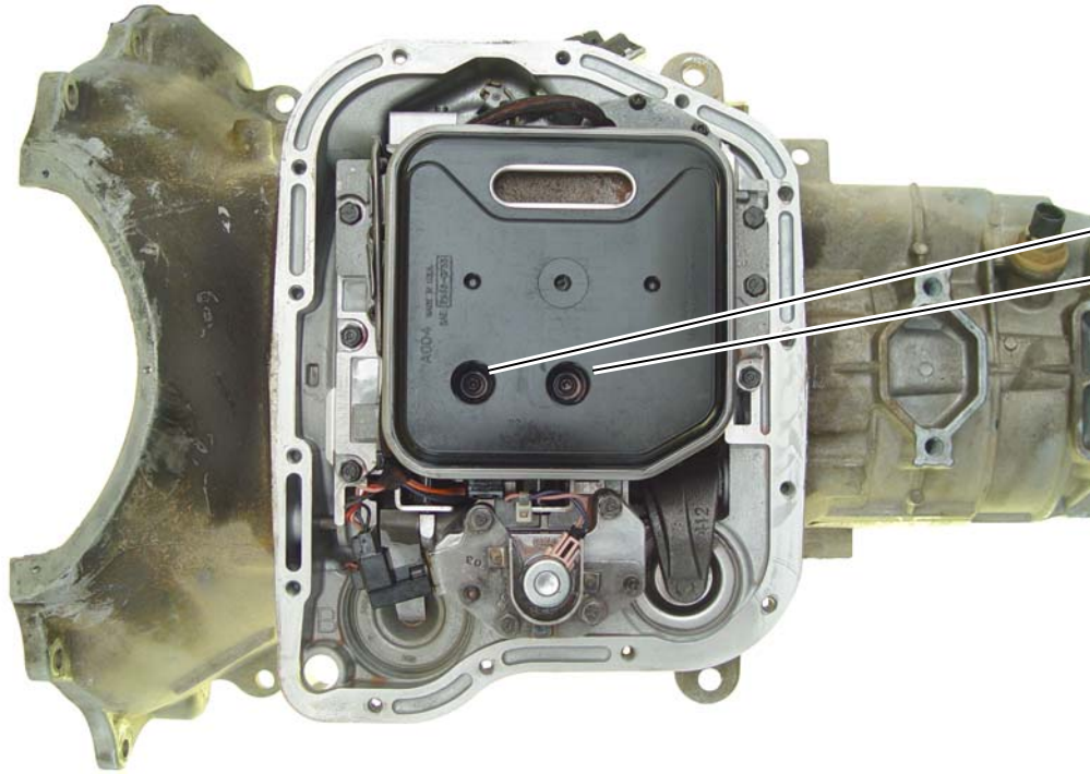
Torx T25 x 2.637" filter screws
